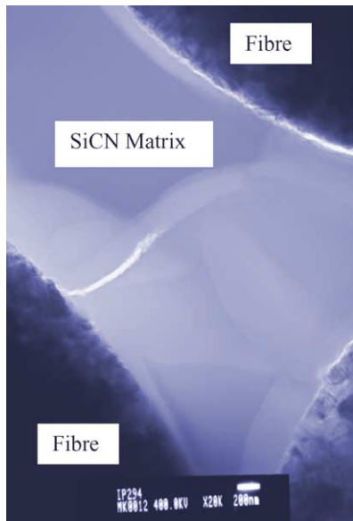
Fig. 5. TEM micrograph showing two matrix regions in a CMC with Ti filler after five PIP cycles.
